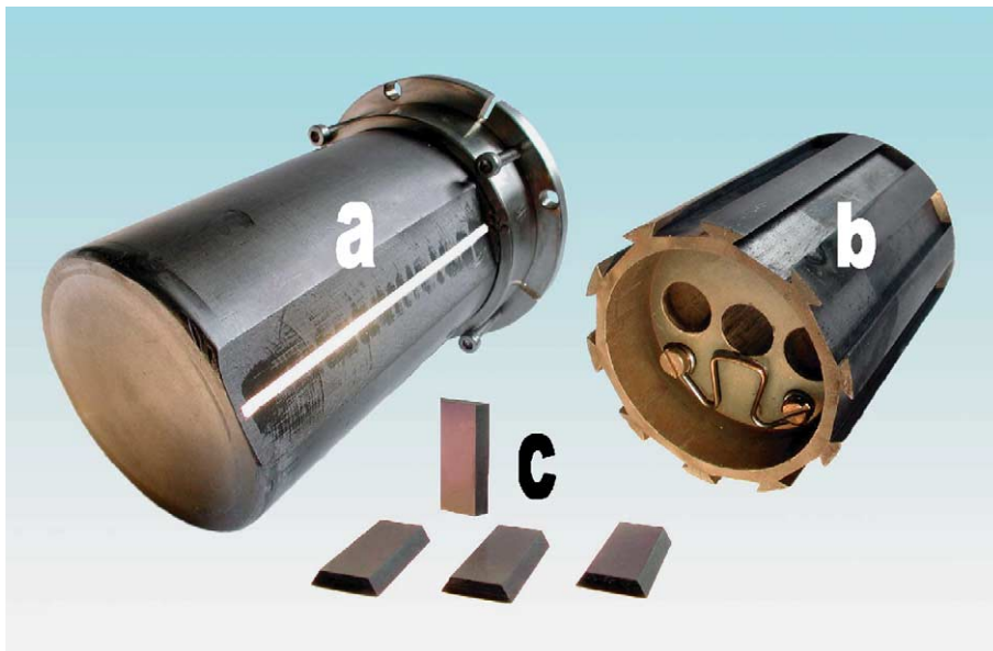
Fig. 1. Surface collector probe: (a) a tantalum housing with 2 mm wide slits, (b) a graphite holder with ten grooves for flux collecting substrates and (c) flux collecting substrates.
